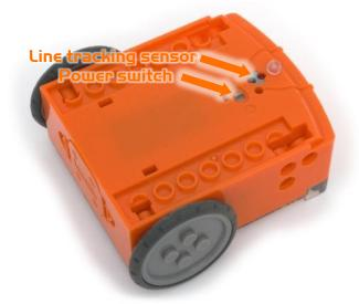
Edison's line tracking sensor is made up of two parts a red LED light and a light sensor. The red LED shines light on the ground, if the ground is white and therefore, reflects light then the light sensor will get a high light reading. If the ground is black and therefore, does not reflect light then the light sensor gets a low light reading.
